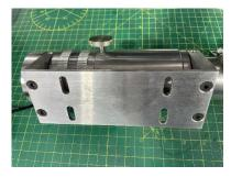
3. Re-fit the screws, however, the screw directly opposite the gearstick must be re-fitted with the longer M4x16 screw provided in the fitting kit.
