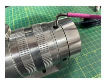
2. Rotate the shifter body to your desired alignment. (If you encounter any resistance do not force it, slacken the 4 base plate screws on the underside of the shifter with a 4mm Allen key).
