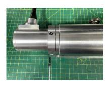
4. Once the shifter is in position, you can amend the orientation of the end cap to suit your wiring configuration by slackening off the grub screw with a 2mm Allen key.
