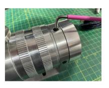
2.Rotate the shifter body to your desired alignment. (If you encounter any resistance do not force it, slacken the 4 base plate screws on the underside of the shifter with a 4mm Allen key).
