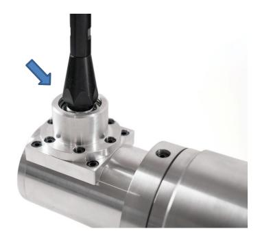
If it looks like the lubrication has dried, the ball joint feels rough or it has been over a year since last adding lubrication after regular use, we recommend smearing a tiny amount (half a pea) lithium-based grease onto the top of the joint and moving through the gears so the parts all get a coating.
