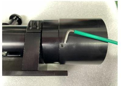
4. Insert the double gate lockout piece as shown.
